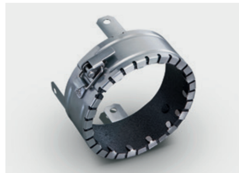
↑ The fire protection sleeve contains an intumescent material which inflates at temperatures of around 150 °C. This inflatable material closes off the feedthrough in the ceiling or behind the wall before the fire and smoke can make their way into other rooms or floors.
